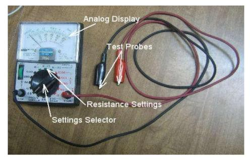
Shown in the figure is an Analog multimeter; it has a pointer moving on a panel like in an ammeter, or a voltmeter.
