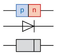
**Forward bias:** When an external voltage is applied to a p-n junction diode in such a way that the p-side is at a higher potential or (is biased to have higher potential) as compared to the n-type.
