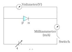
Circuit Diagram for forward Bias Characteristic Curves
